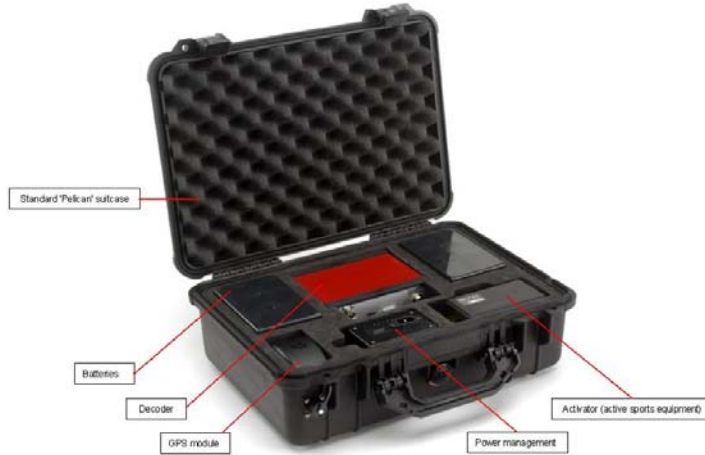
Image 1: Overview Track Side Box
