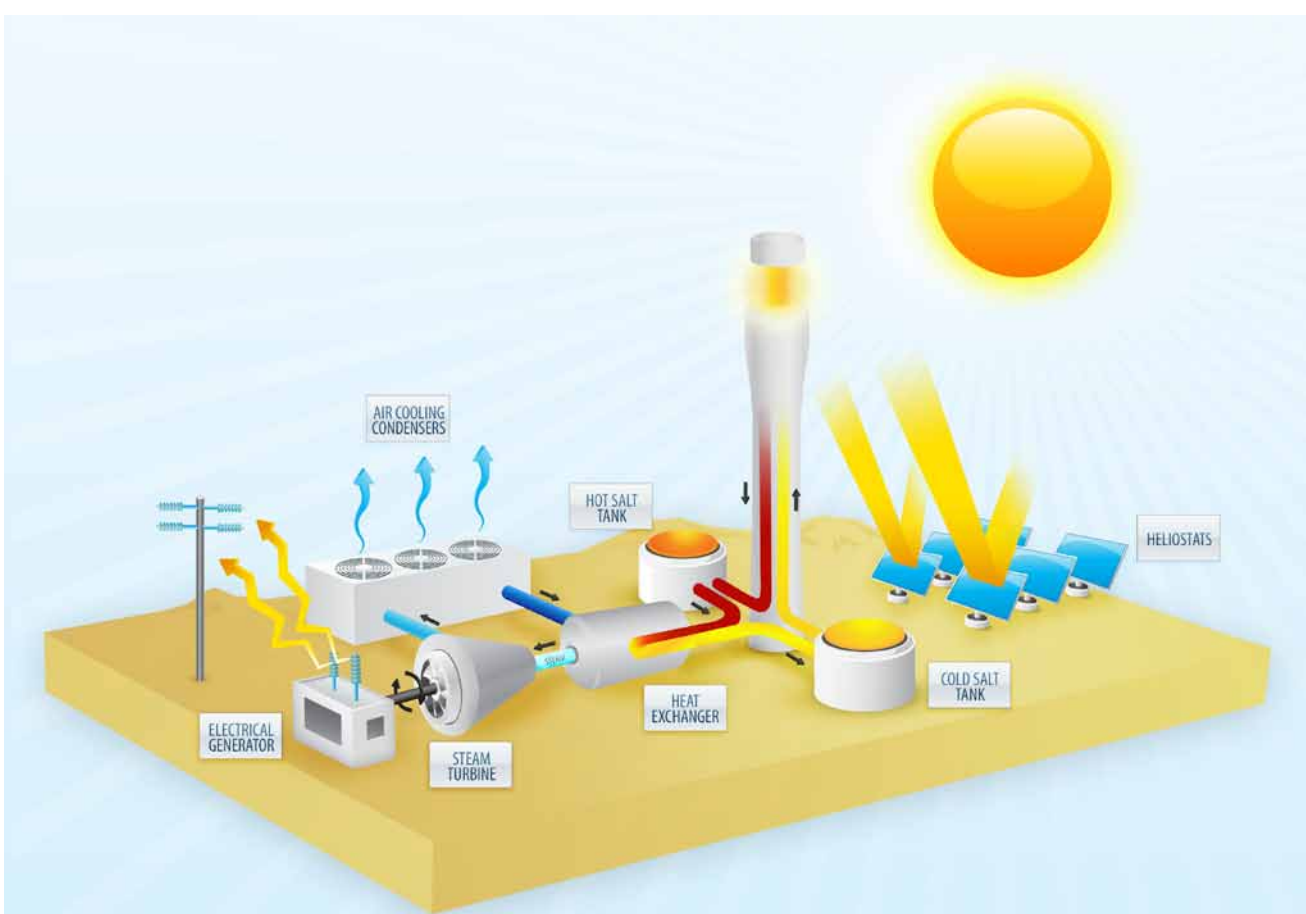
FIGURE 7 Solar Thermal Power Tower
