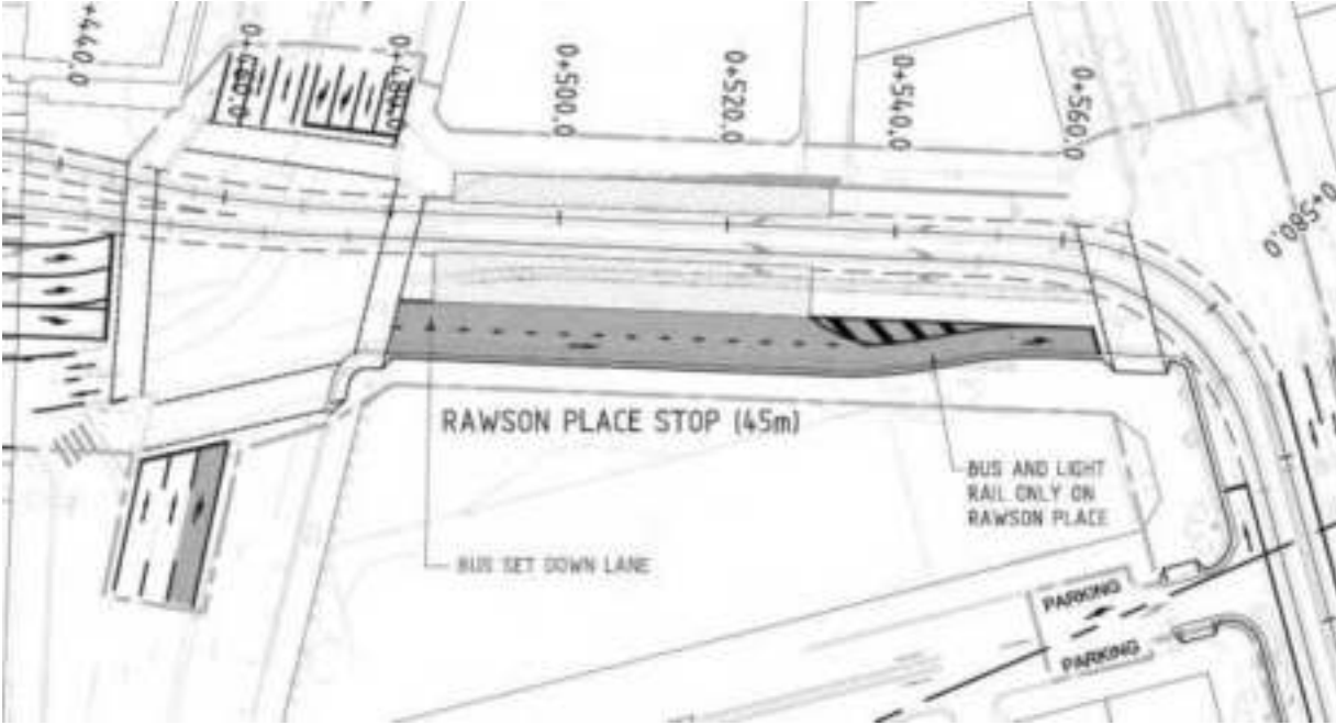
Figure 7-8: Rawson Place Interchange Design
