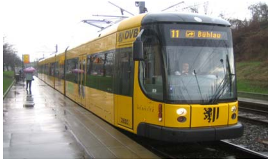
City tram of Dresden – with more than 45 metres the longest in the world
